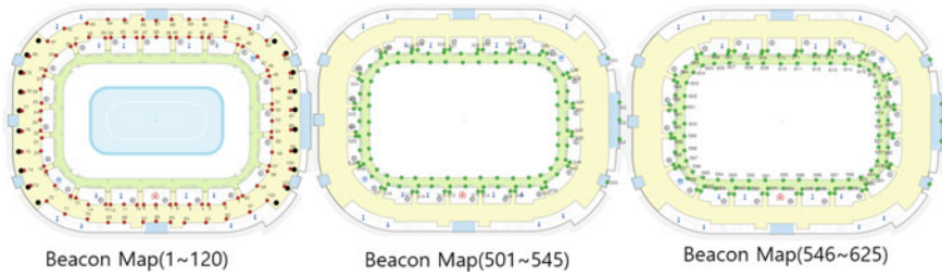
Fig. 12 Location of BLE beacons:125 beacons at 1st floor, 166 beacons at 2nd floor including corridor or crowded places
